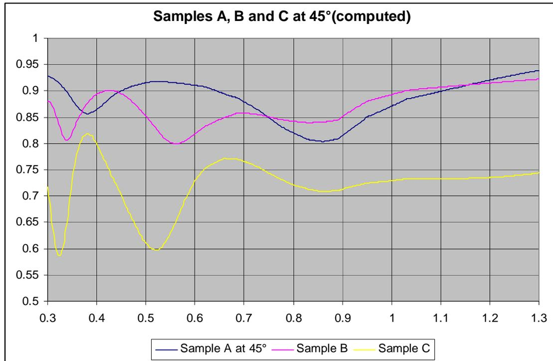
Fig. 3 Computed reflectivity of the three samples at 45° incidence.
