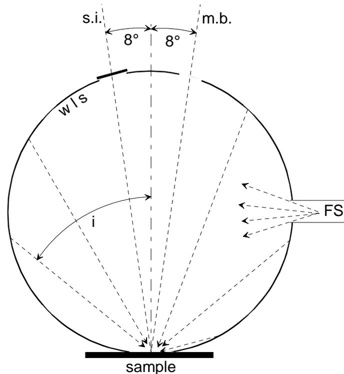
Fig. 7 Optical structure of the MNLT albedo meter.
