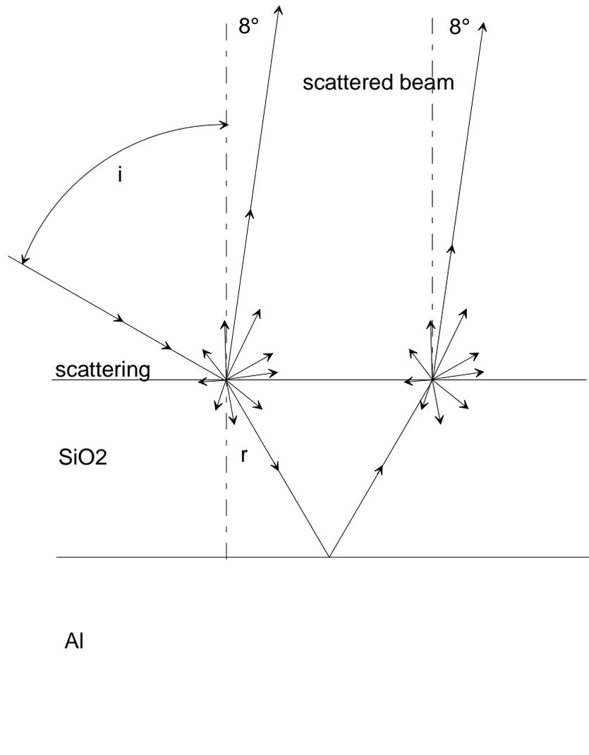
Fig. 8 Light reflection and scattering on a SiO<sub>2</sub> over coated Al coating
